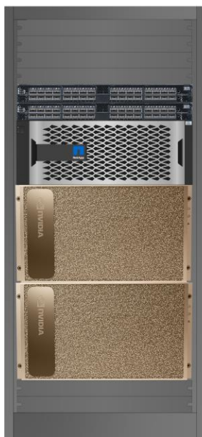
2 DGX A100 systems 1 AFF A400 storage system 2 SN3700V switches
